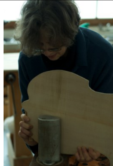
ill. 18: heat-bending the back, photo: N. P. Stefanovitch
