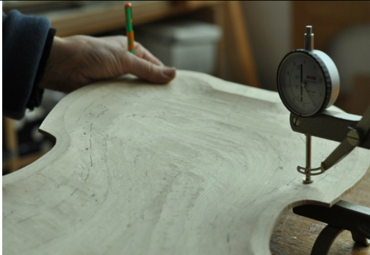
ill. 5: front inside with the mapped-out thicknesses, photo: Nemo Perier Stefanovitch
