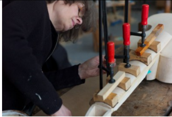
ill. 41: gluing the fingerboard, photo: N. P. Stefanovitch
