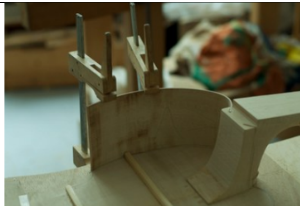
ill. 29: top rib glued into the neck block and to the back, photo: N. P. Stefanovitch
