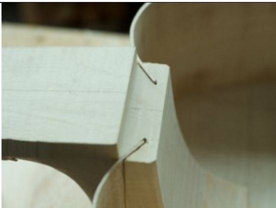
ill. 28: top ribs inserted into the neck block, photo: N. P. Stefanovitch
