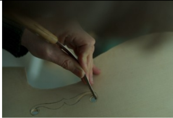
ill. 35: cutting soundholes, photo: N. P. Stefanovitch
