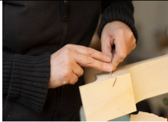
ill. 15: filing the rib slots, photo: N. P. Stefanovitch
