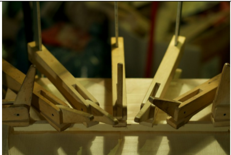
ill. 20: gluing the back ribs, photo: N. P. Stefanovitch
