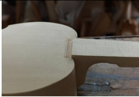
ill. 38: purfling under the fingerboard, photo: N. P. Stefanovitch
