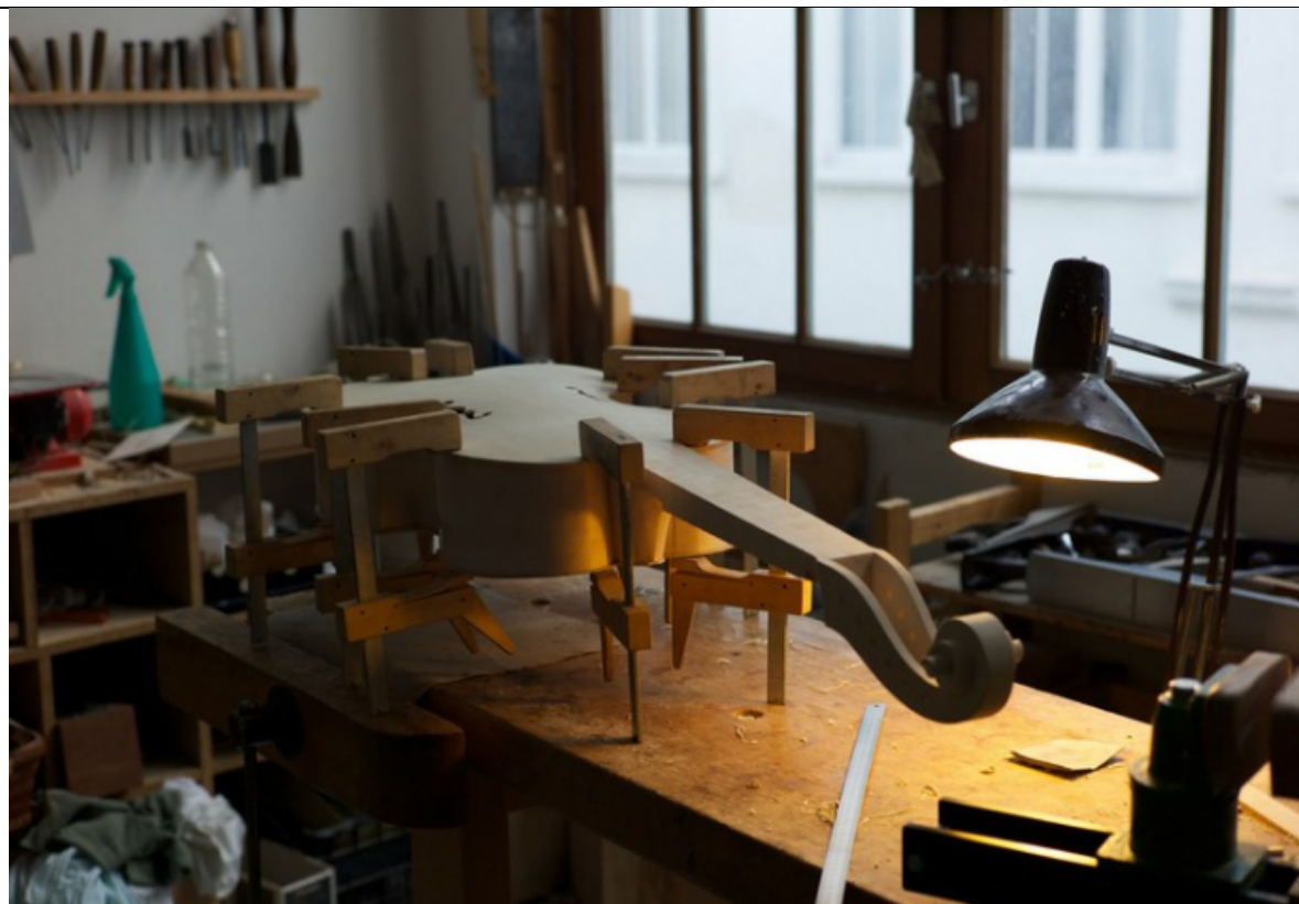
ill. 36: gluing the front, photo: N. P. Stefanovitch
