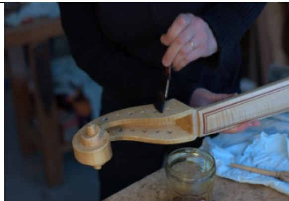
III. 45: varnishing the pegbox, photo: N. P. Stefanovitch
