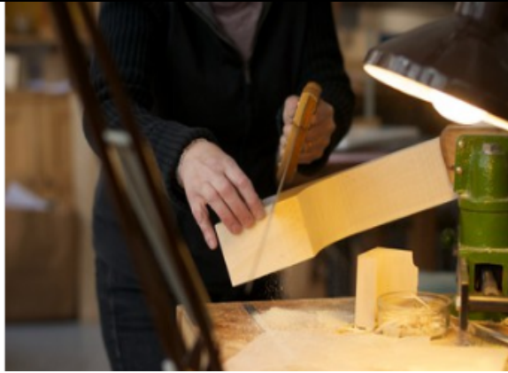
ill. 14: sawing the rib slots, photo: N. P. Stefanovitch
