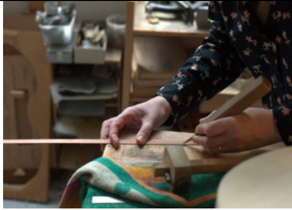
ill. 37: cutting the purfling, photo: N. P. Stefanovitch
