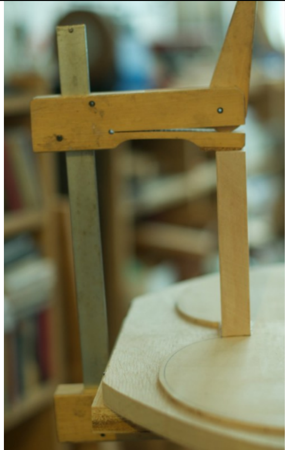
ill. 22: gluing the bottom block to the back, photo: N. P. Stefanovitch
