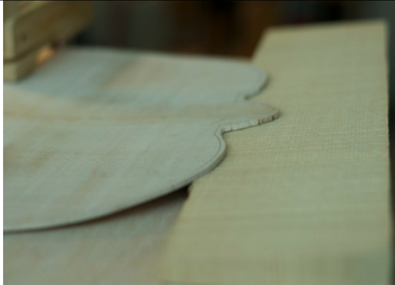
ill. 17: bending the back by force, photo: N. P. Stefanovitch
