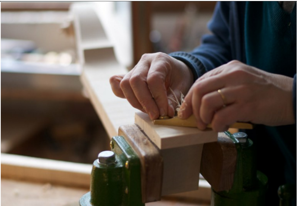
ill. 16: shaping the curve of the heel foot of the neck, photo: N. P. Stefanovitch
