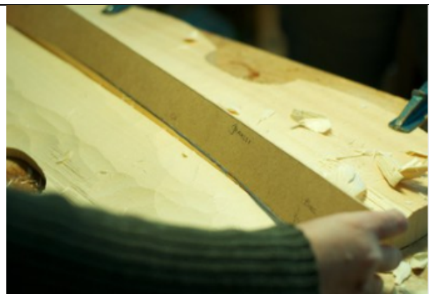
ill. 4: front with arching template, photo: N. P. Stefanovitch
