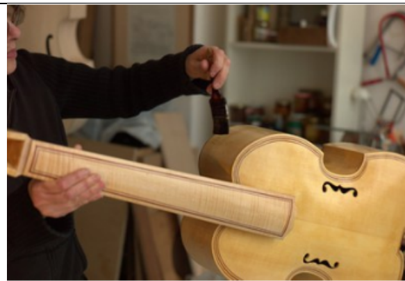
III. 44: varnishing the ribs, photo: N. P. Stefanovitch
