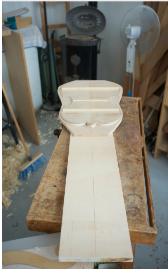
ill. 21: gluing structure with the back attached, photo: N. P. Stefanovitch
